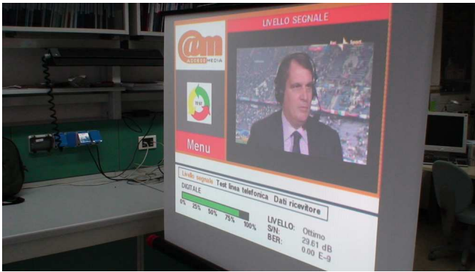
Fig. 5. Output of the Access Media STB1230 test receiver fed by the Soft-DVB transmitted signal.
